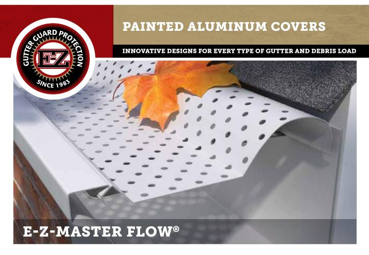
This effective and simple-to-install aluminum gutter guard has our highest level of engineering to date — with perforations and an arched rear, this recessed cover works with both types of hangers. The arched rear assists debris forward and water downward through the perforated holes.
