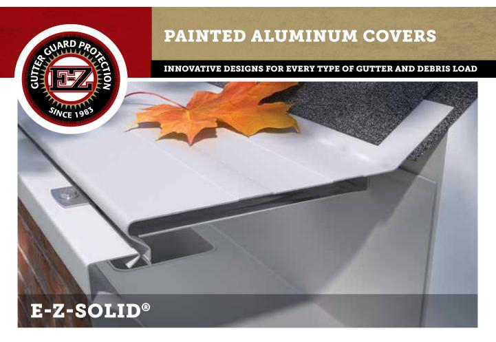
This solid guard allows the water to track around the front (by surface tension) and into the gutter, while forcing debris to fly off. The clips install first and maintain a consistent gap along the leading edge, so water tracks around the patented-design multiple radius curve and into the gutter. It also features a perforated bend line where the metal meets the roof. We also supply diverters for use in valleys.
