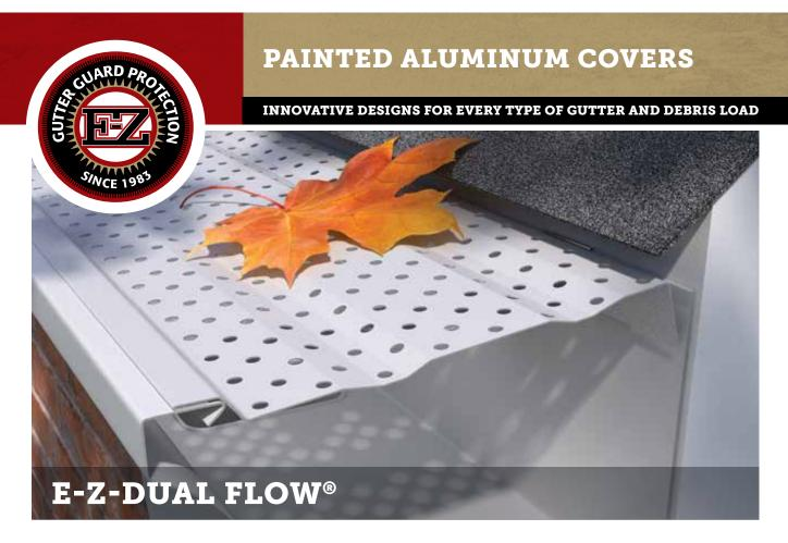
This effective and simple-to-install aluminum gutter guard recesses into the gutter and fastens to the front with stainless steel screws (provided). With thousands of holes, the rain water passes through the canals, making it E-Z for air flow to dry the debris and blow it away.
