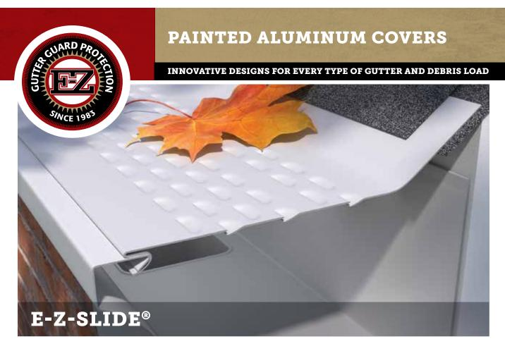
This cover works with all gutter systems, and installs between shingles, fastening into the top front of the gutter with stainless zip screws provided. It features 6 rows of our patented reverse-louvers, and bends to conform to the pitch of the roof and the fall of the gutter. Water drops into the gutter and debris slides over the front of the gutter.
