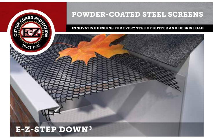
This design works for every gutter installation, with spring tension that holds it in place, while closing the void under the shingles so debris can't collect there. It is one of the few guard systems available today that snaps in and out for easy cleaning. The steel is .028 – to stand tough under a full load of wet leaves without collapsing – and installs with a slope toward the front to help debris slide off.
